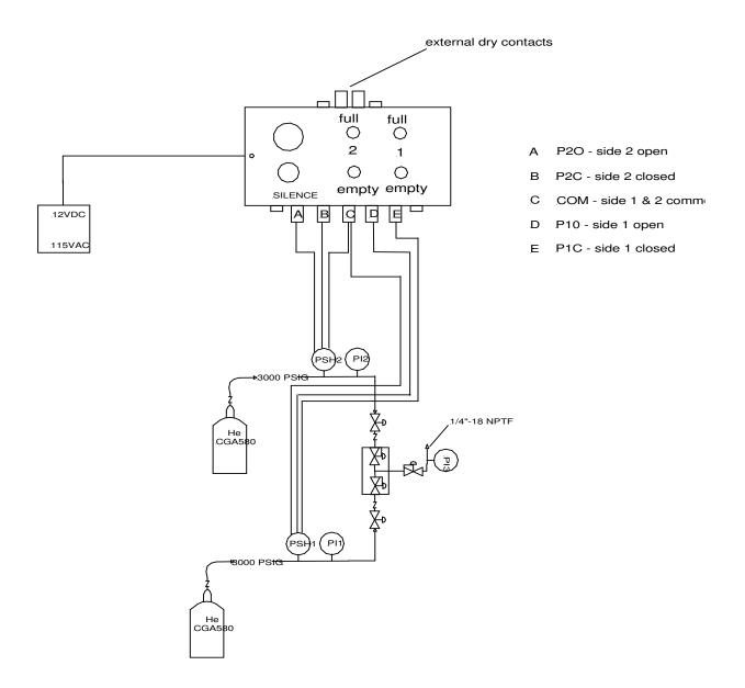
PSH1, PSH2 PRESSURE SWITQH1,PI2 PRESSURE GAUGE I 3, PRESSURE GAUGE SET POINT@ 300 +/- 25 PSIG 3000 PSIG 200 PSIG
